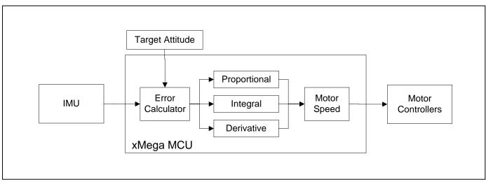
Figure 3. Attitude Control Diagram
