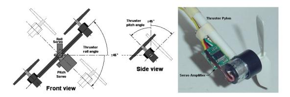
Figure 3. Propulsion thrust vector control.
