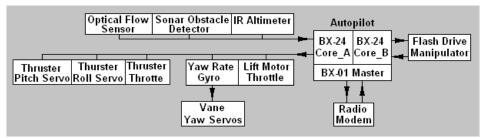
Figure 5. Control system architecture.
