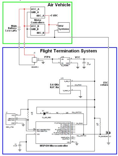
Figure 6. Flight termination system.
