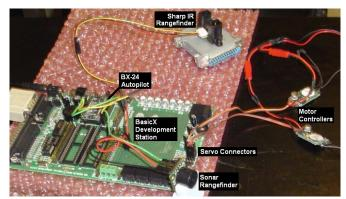
Figure 9. Autopilot breadboard with sensors.
