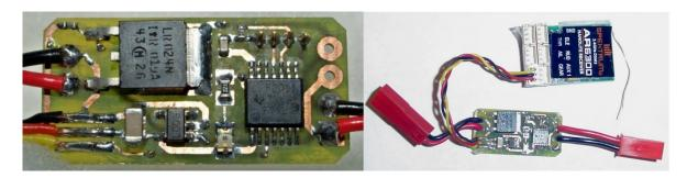
Figure 7. Flight Termination System board (left). Board with radio receiver (right).
