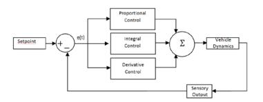
Figure 3 - Control Loop Architecture
