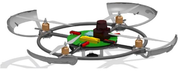
Figure 2 - MAAVerick Structure and Electronics
