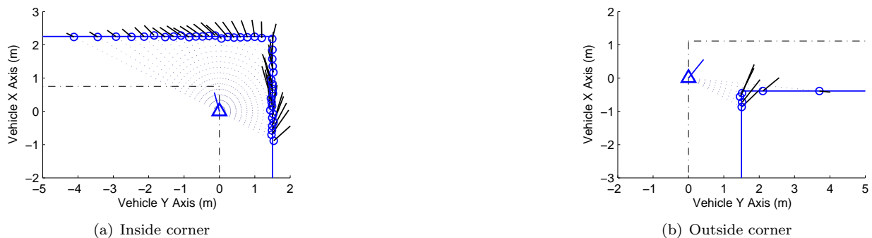
Figure 4. Inside and outside corners are handled with no special topology check required. The average velocity vectors generate a total commanded velocity that takes the vehicle smoothly through the maneuver. Heading commands are generated to turn the vehicle parallel with the next wall face as soon as it is detected.
