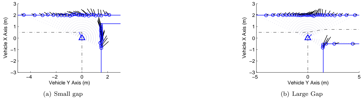
Figure 5. Any gap in the wall is detected by the PRLS wall estimation algorithm. Gaps that are smaller than the desired threshold are flown by with no effect on the commanded velocity. Gaps that are large enough for the vehicle to fly through, such as a hallway or door, cause the commanded velocity vector to bend toward the opening. If the vehicle enters a hallway or goes through a door where the minimum lateral separation is not at least twice the wall follow distance, the vehicle simply keeps an equal distance from both sides. Otherwise, the vehicle picks up the wall on the right hand side and keeps the desired distance from it as flight continues.
