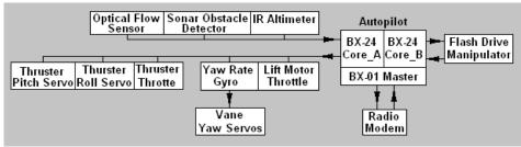
Figure 5. Control system architecture.
