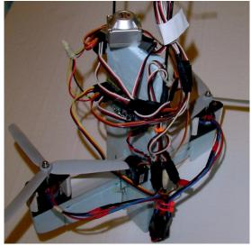
Figure 4. Gondola with lift fans and vanes.
