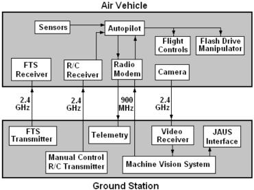
Figure 1. Overall system architecture.
