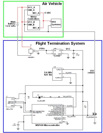
Figure 6. Flight termination system.
