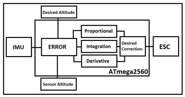
Figure 2. Simplified PID Logic Flow Diagram
