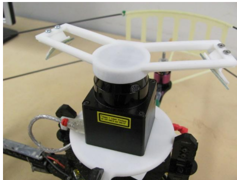
Figure 5: LIDAR mirror mount for height estimation
