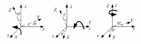
图 2-4 滚动、俯仰和偏航示意图 Fig.2-4 Rotations in roll, pitch and yaw
