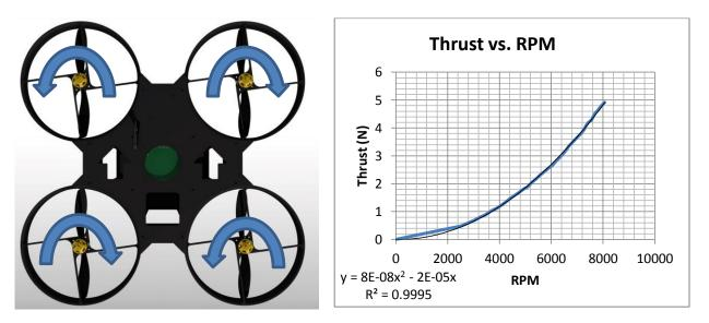
Figure 2: a) Rotor configuration b) Thrust vs. RPM curve for motor/propeller combo
