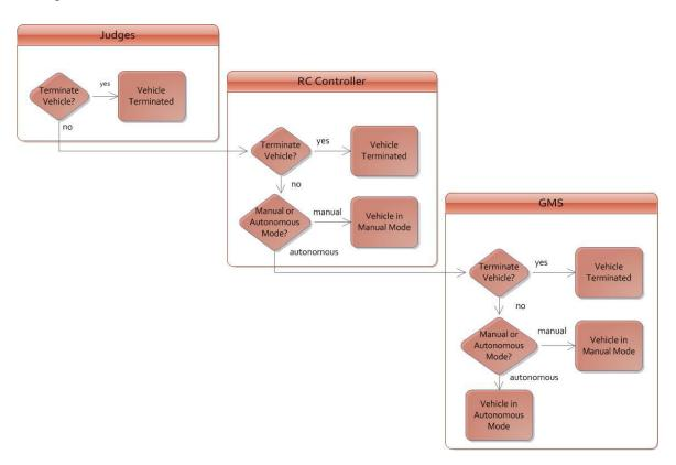
Figure 4: Man/Machine Interface Command Hierarchy
