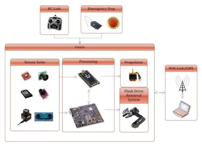
Figure 1: ERAU Raven System Architecture
