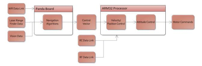
Figure 3: Control System Architecture
