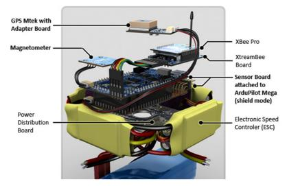
Fig.4 Auto-Pilot System Layout
