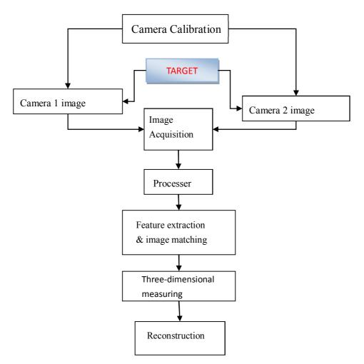
Fig.2 Camera system Module
