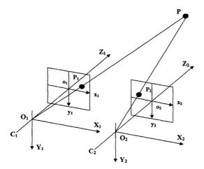
Fig.3 Binocular vision system calibration
