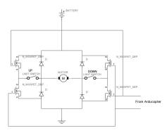
Figure 8: H-Bridge circuit drawing.
