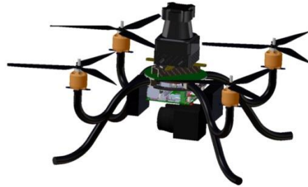
Figure 9: A model in CATIA V5. This was used for full vehicle fabrication and assembly (left) Simulation for path planning algorithms and vehicle stability testing (right)
