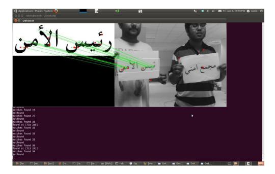
Figure 6 : SURF Bruteforce Matching via RANSAC
