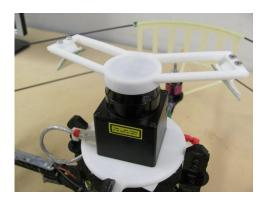
Figure 5: LIDAR mirror mount for height estimation
