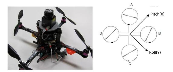
Figure 2: The Asctec Pelican quadrotor and the propeller action.
