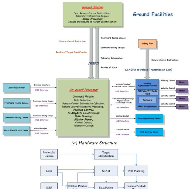
(b) Algorithm Interaction Figure 1. Overall System Architecture
