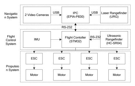
fig2.2 System hardware structure
