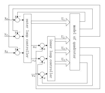
fig2.4 Structure of the double loop PID control system
