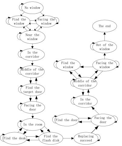
fig2.7 The state transition diagram of the mission
