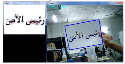
fig2.6 A sign recognized using SURF
