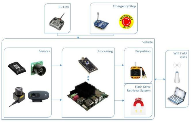
Figure 1: ERAU Raven II System Architecture
