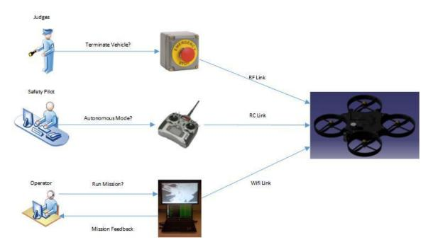
Figure 5: Man/Machine Interface Hierarchy
