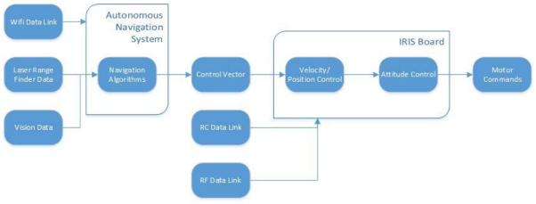
Figure 4: Control System Architecture
