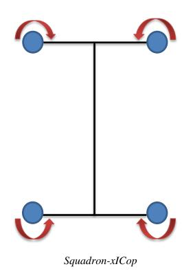
YAW ANGLE: The angle between an aircraft's longitudinal axis and its line of travel, as seen from above. Left yaw is achieved in Squadron-xIcop when rpm of the motors 2 and 4 increases and rpm of motors 1 and 3 are at normal. Right yaw is achieved when rpm of the motors 1 and 3 increases and rpm of the motors 2 and 4 are at normal.
