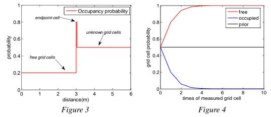
Figure 3 shows the probability of grid cells in a beam direction. Distance of the beam is 3 meters.  $P_{free} = 0.2$  and  $P_{occ} = 0.8$ . Figure 4 shows the change of probability when a grid cell is measured several times as free or occupied.
