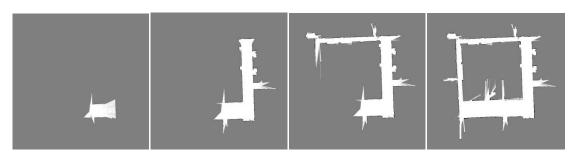
*Figure 7. Incremental mapping of New Main Building of Beihang University. The left image shows the initial map and the right image shows the resulting map.*
