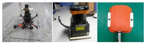
Figure 5. Our quadrotor platform (left), UTM-30LX laser range finder (middle) and XSens IMU (right).
