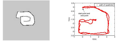
Figure 6. Map of Tsinghua experimental site (left) obtained in real time using our algorithm, and the trajectory of our quadrotor (right) after closing the major loop.
