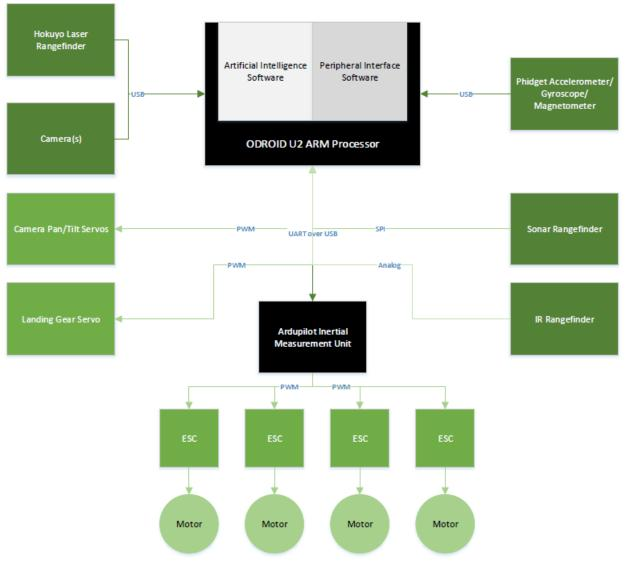
Figure 1. Control System Architecture.
