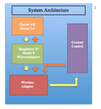
Figure 2, System Architecture of APUS
