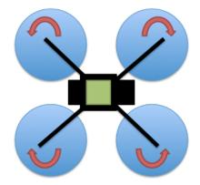
Figure 1, Motor Configuration of the Vehicle
