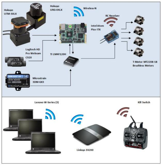
Figure 2: MAAV System Architecture
