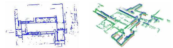
Figure 3: (left) 2D map generated with only a horizontal laser, (right) 3D map generated with both vertical and horizontal lasers
