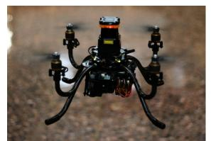
Figure 1: A front shot of the MAAV quadrotor fully assembled
