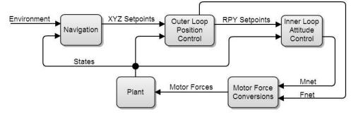
Figure 4: Control scheme diagram
