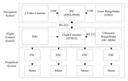
Fig2.2 System hardware structure
