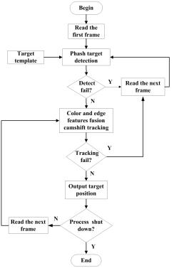
Fig2.6 Ground target tracking algorithm
