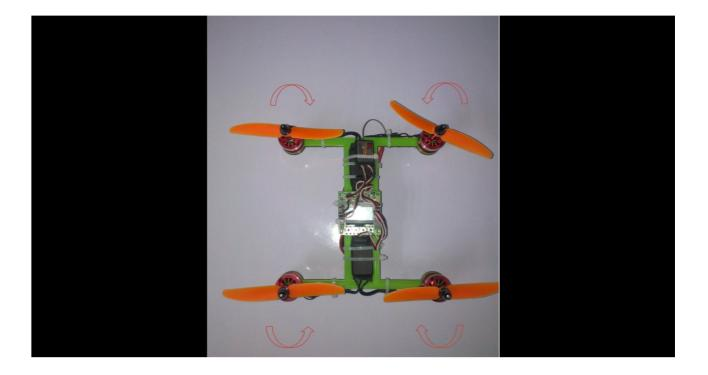
YAW ANGLE: The angle between an aircraft's longitudinal axis and its line of travel, as seen from above. Left yaw is achieved in Squadron II when rpm of the motors 2 and 4 increases and rpm of motors 1 and 3 are at normal. Right yaw is achieved when rpm of the motors 1 and 3 increases and rpm of the motors 2 and 4 are at normal.
