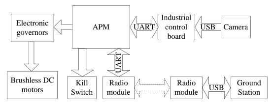
Figure 1. Hardware structure diagram of unmanned quadrotor helicopter
