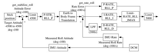
Figure 4. Structure diagram of roll controller
