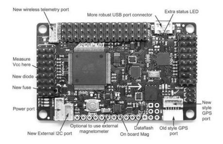
Figure 2. Flight control board
