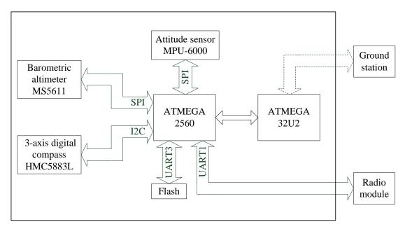
Figure 3. Interface diagram of APM
