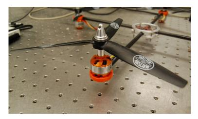
*Figure 3: Initial motor mount configuration. The longer moment arm made the mount prone to vibrations.*
