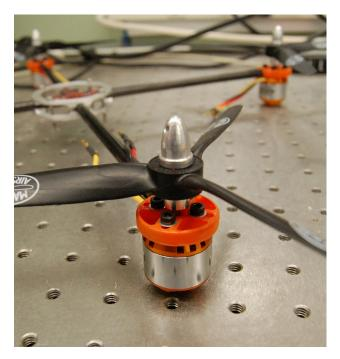
*Figure 4: Final motor mount configuration. Having the two rotating masses on either side of the mount reduces vibration.*
