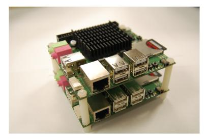
*Figure 6: Stack of two Odroids.*
