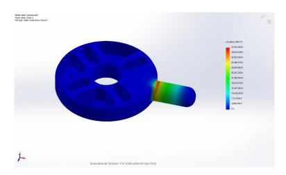
*Figure 2: FEA with red indicating high levels of stress. Forces applied torsionally simulating torques from Figure 3.*
