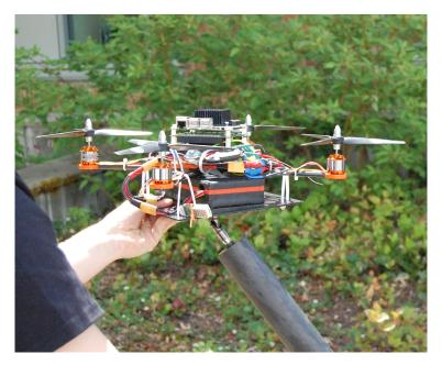
Figure 9: Quadrotor on test mount.
