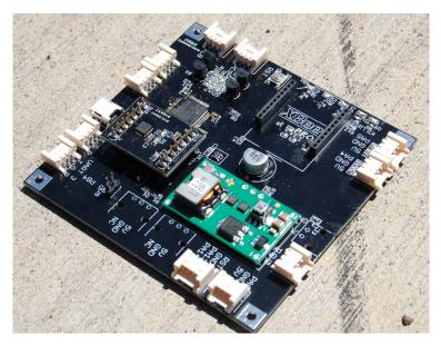
Figure 7: The latest revision of the flight control board.
