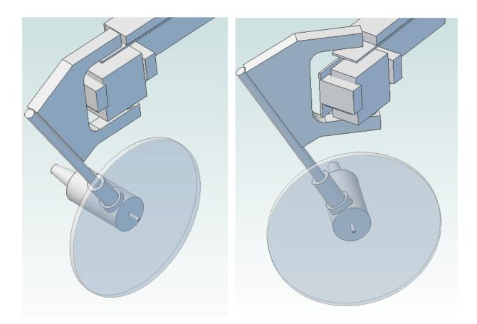
Figure 3. Propulsion thrust vector control. At left, thruster is centered. At right, thruster is deflected 45°.
