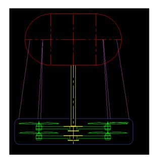
Figure 9. This image is a symbolic representation of the following components: balloon (red), propellers (green), cage (blue) and strings/rods (purple).
