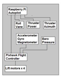
Figure 5. Control system architecture.
