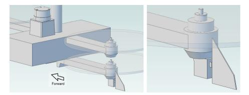
Figure 4. Aft roll vane.
