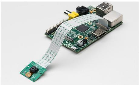
Figure 6. Raspberry Pi with camera.
