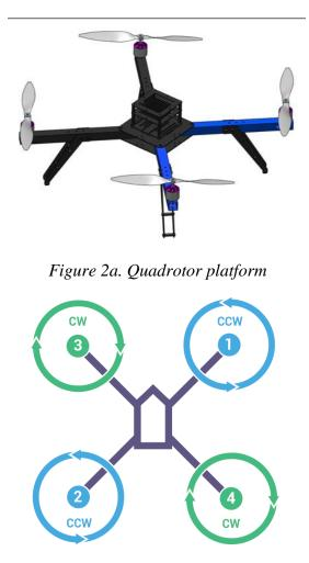
Figure 2b. Quadrotor propulsion system
