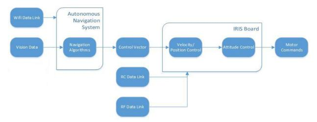
Figure 3: Control System Architecture
