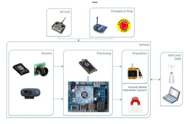
Figure 1: ERAU RAVEN II System Architecture
