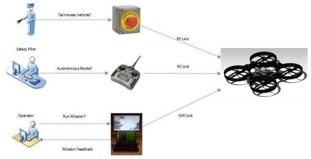
Figure 4: Man/Machine Interface Hierarchy
