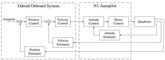
Figure 3. Control system architecture
