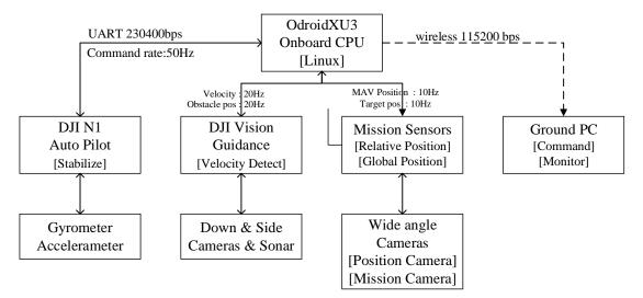
Figure 1. The overall system architecture
