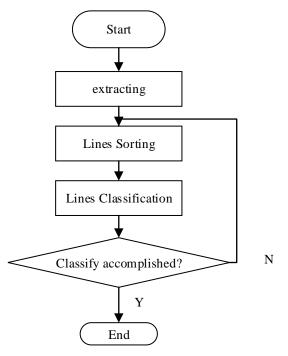
Figure 4. Lines filtering algorithm
