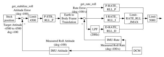
Figure 4. Structure diagram of roll controller
