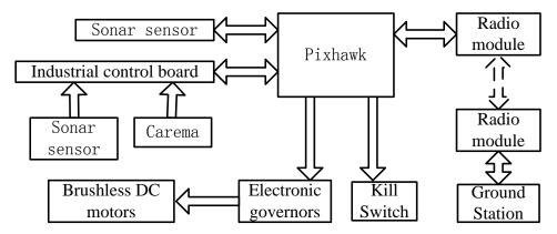
Figure 1. Hardware structure diagram of unmanned quadrotor helicopter
