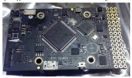
Figure 2. Flight control board
