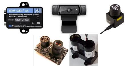
Figure 3: From left to right and top to bottom, The Microstrain 3DM-GX3-25, Logitech C920 Webcam, Hokuyo URG-04LG-UG01 Laser Rangefinder, PX4 Optical Flow Sensor, and Pulsed Light Lidar-Lite Laser Module
