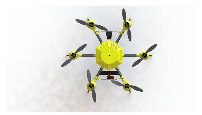
Figure 2: A render of the top view of the multirotor airframe.
