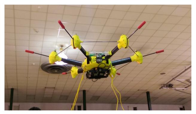
Figure 4: An autonomous flight test conducted with safety tethers attached.
