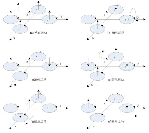
Figure 6. The quad-rotor along the various degrees of freedom of movement.
