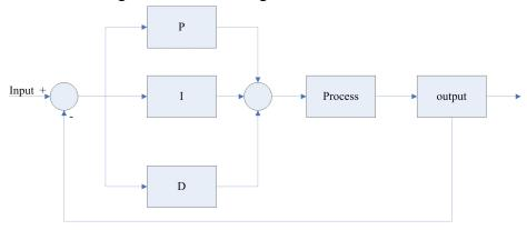
Fig.3 PID control block diagram
