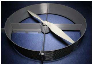
Figure 6. Ducted Propeller
