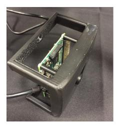
Figure 6. ELP camera at left. At right is the camera mounted in 3D printed cage with Raspberry Pi computer
