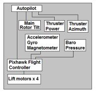
Figure 3. Control system architecture.
