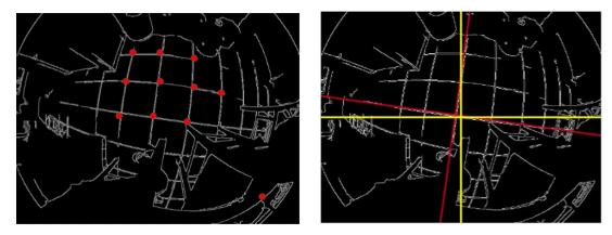
Figure 8. Grid detection using corner detection (left) and Hough transforms (right)
