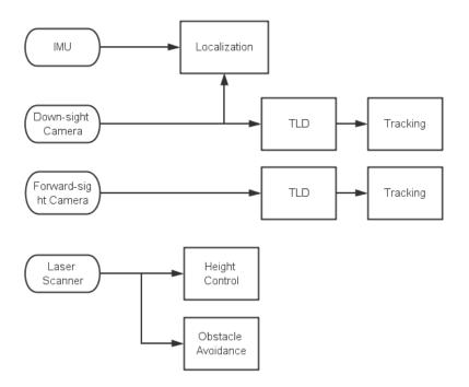
Figure 4: The Software Structure in Searching Mode
