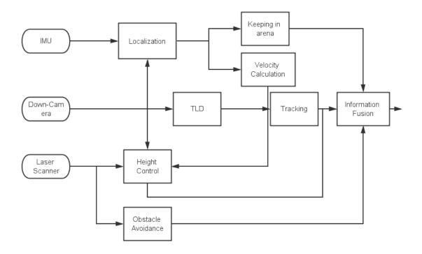
Figure 3: The Software Structure in Herding Mode
