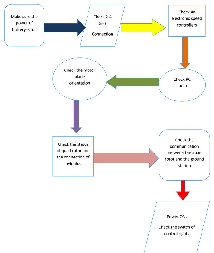
The following checklists are carried out after performing the initial setup and visual checks
