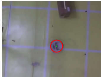
Bot Detection using Ellipse Detection for downward facing camera
