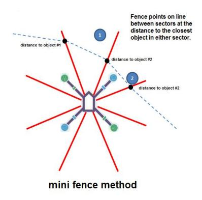
Figure 4. Mini Fence Method for Object Avoidance
