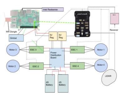
Figure 6. Wiring Diagram
