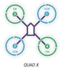
Figure 3. Quadrocopter motor layouts
