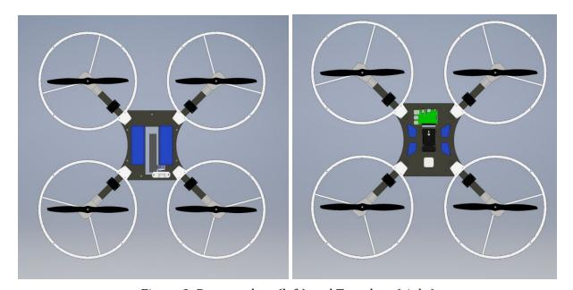
Figure 2. Bottom plate (left) and Top plate (right)
