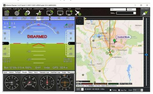
Figure12.Man/Machine Interface Diagram
