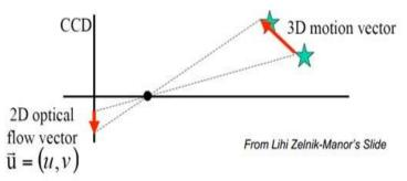
Figure 4. Sketch Diagram of Optic Flow Field and Motion Field
