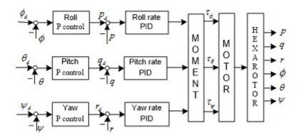
Figure3. The Detail of Attitude Control Block
