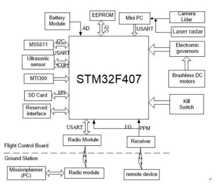
Figure 5. Control System Architecture (Hardware)
