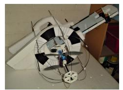
Figure 9. Vehicle in inverted takeoff orientation.
