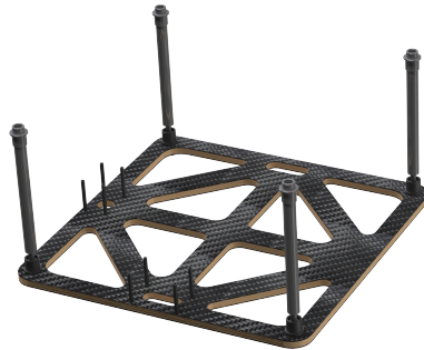
Figure 6. New landing gear for robot interaction.
