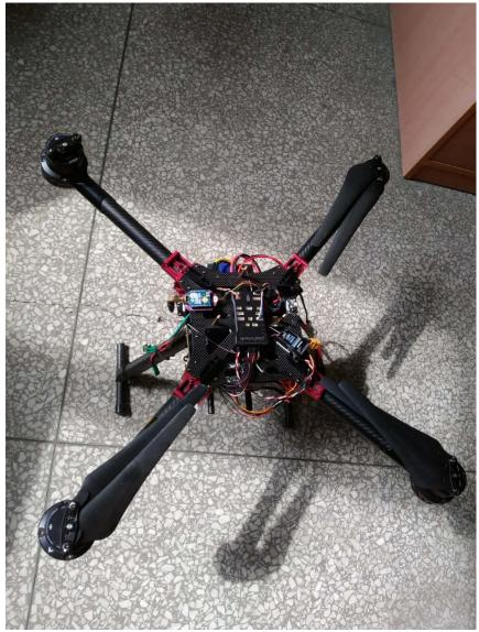
Figure 2. Flight platform of THBOT
