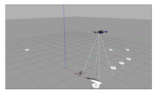
To simulate the quadcopter, we use Ardupilot's Software in the Loop (SITL) simulation method to run a Gazebo simulation with ROS. Using the PX4 flight stack, we are able to simulate a quadcopter like ours with a Pixhawk and Optical Flow sensor.
