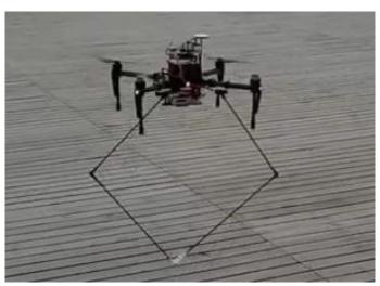
Figure 5: Parallel Mechanical Arm
