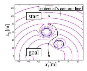
Figure 12: Artificial potential field approach
