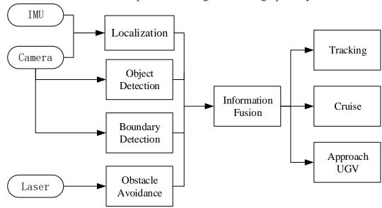
Figure 7: AGV system structure
