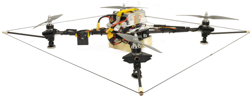
Figure 2. Image of the drone showing the frame, target bumpers, propulsion, batteries, and landing gear.
