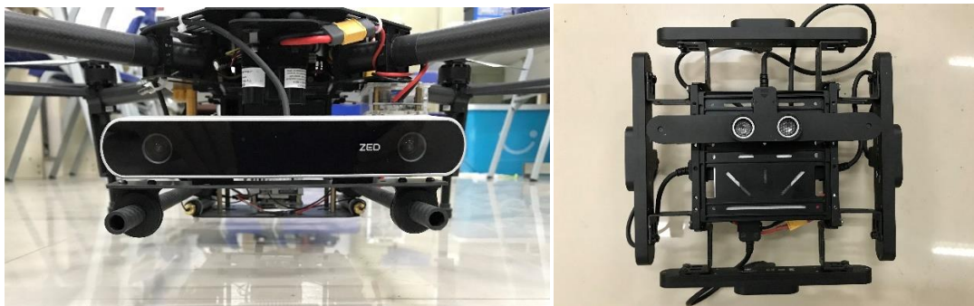
Figure 6. ZED Stereo Camera and DJI Guidance system
