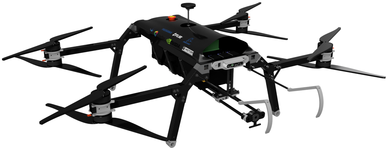
Figure 1. 3D model of competition aerial vehicle. The claws located in the front are meant to remove the existing antenna module from the mast.
