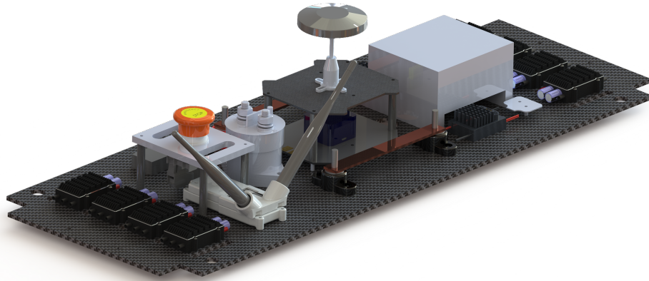
Figure 2. Model of layout of onboard electronics
