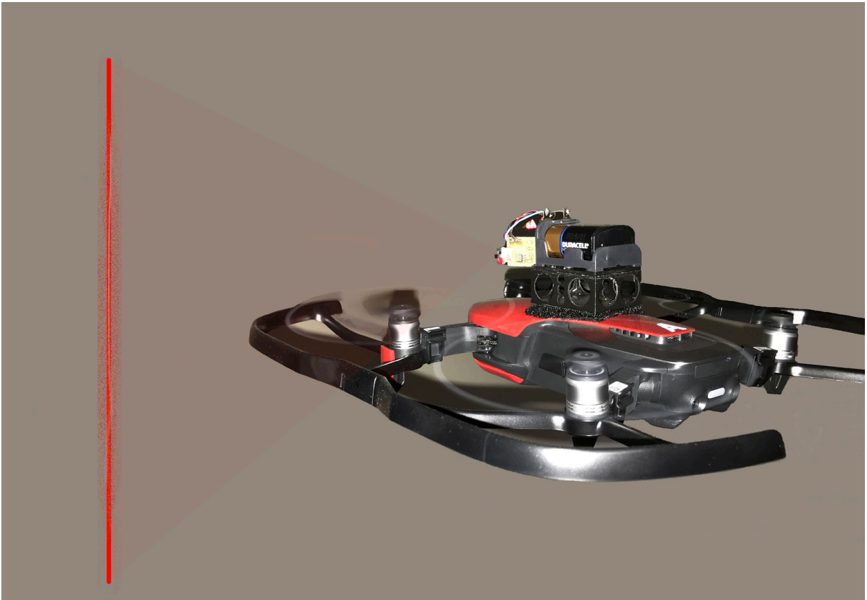
Mavic Air Sentry with laser carriage and riser mounted to upper surface with velcro.
