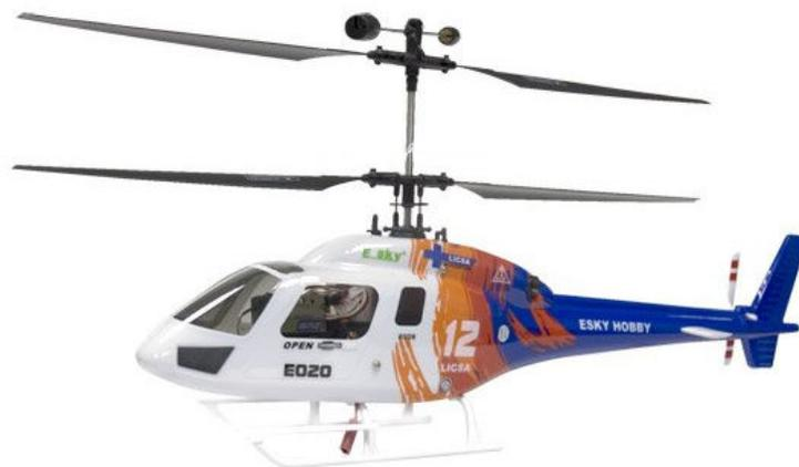
**Figure 1** The Esky E020 “Big Lama” coaxial helicopter. Note: the tail rotor on this aircraft is neither functional nor required for flight.
